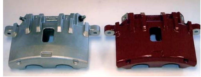
High Performance Brake Blasted with Zinc Cut Wire & Prior to Blast
